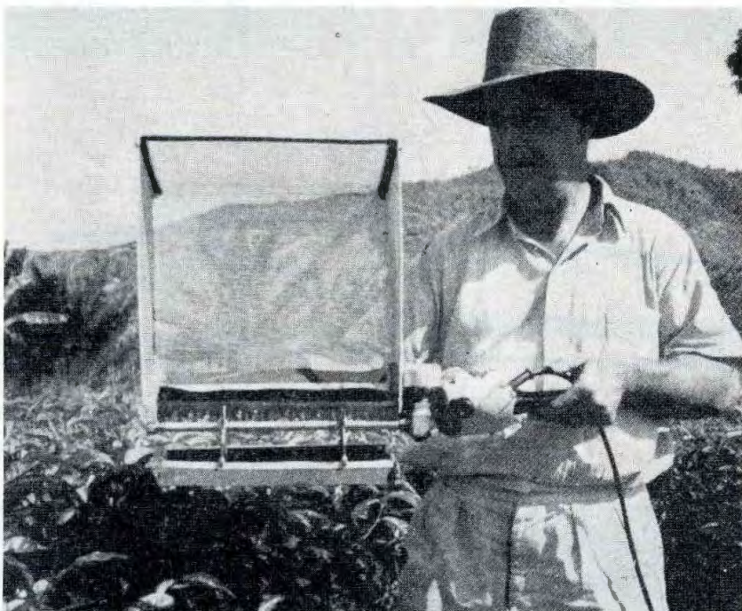
Tea Harvesting Partly Mechanised. An individual cutting unit is here up-ended to show gauze container on top, cutter-bar and reel at bottom, and electric motor and carrying handles on right.
